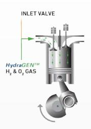
HydraGEN<sup>M</sup> delivers the optimal ratio of H<sub>2</sub> and O<sub>2</sub> to the engine's air intake port during the intake stroke.
